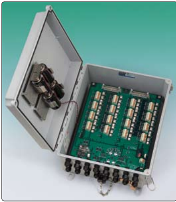
● Model 8002-16-1 (LC-2x16) 16-Channel Datalogger opened to show interior detail.
