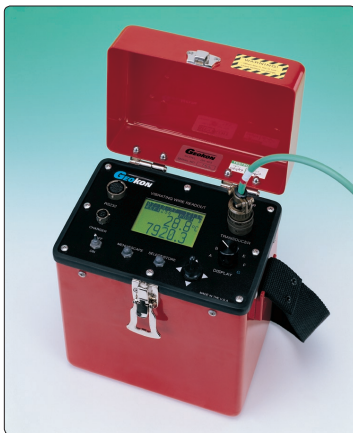
● Geokon Model GK-403 Readout Box for use with the Model 4000 and 4050 Strain Gages.
